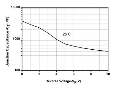
Fig.3-Capacitance vs. Reverse Voltage
